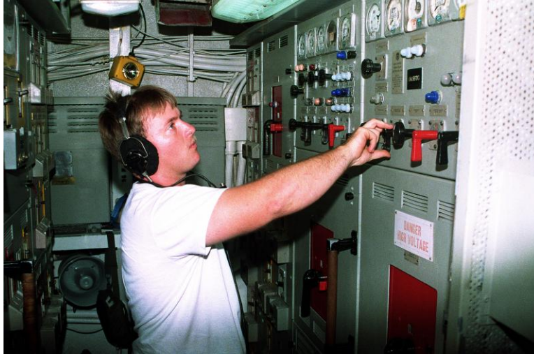
Figure 3: USS Goldsborough (DDG 20) Ship Service Switchboard (Public Domain)
